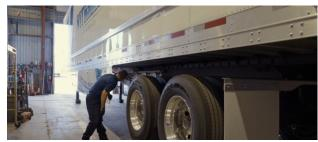
After treatment, walk around trailer for inspection. If it's leaking you will see white bubbles from piping. Close main valve, drain the tanks.
